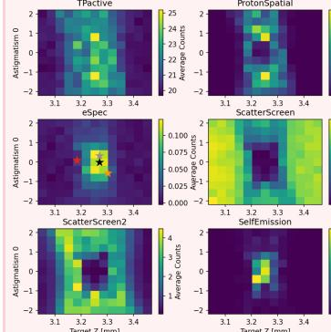
Slices of parameter space mapped with grid scans provide valuable insight (left: target position vs. astigmatism) but are inefficient for multi-dimensional parameter space.
