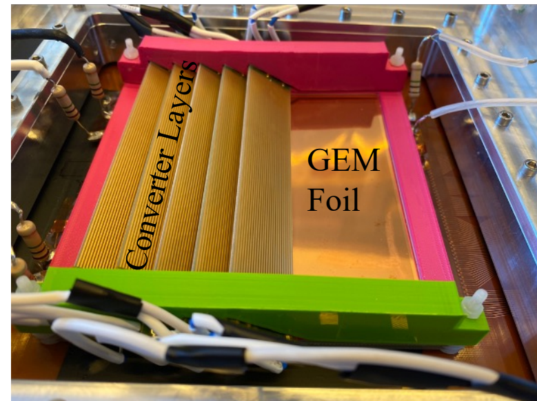
multiple converter layers in detector
