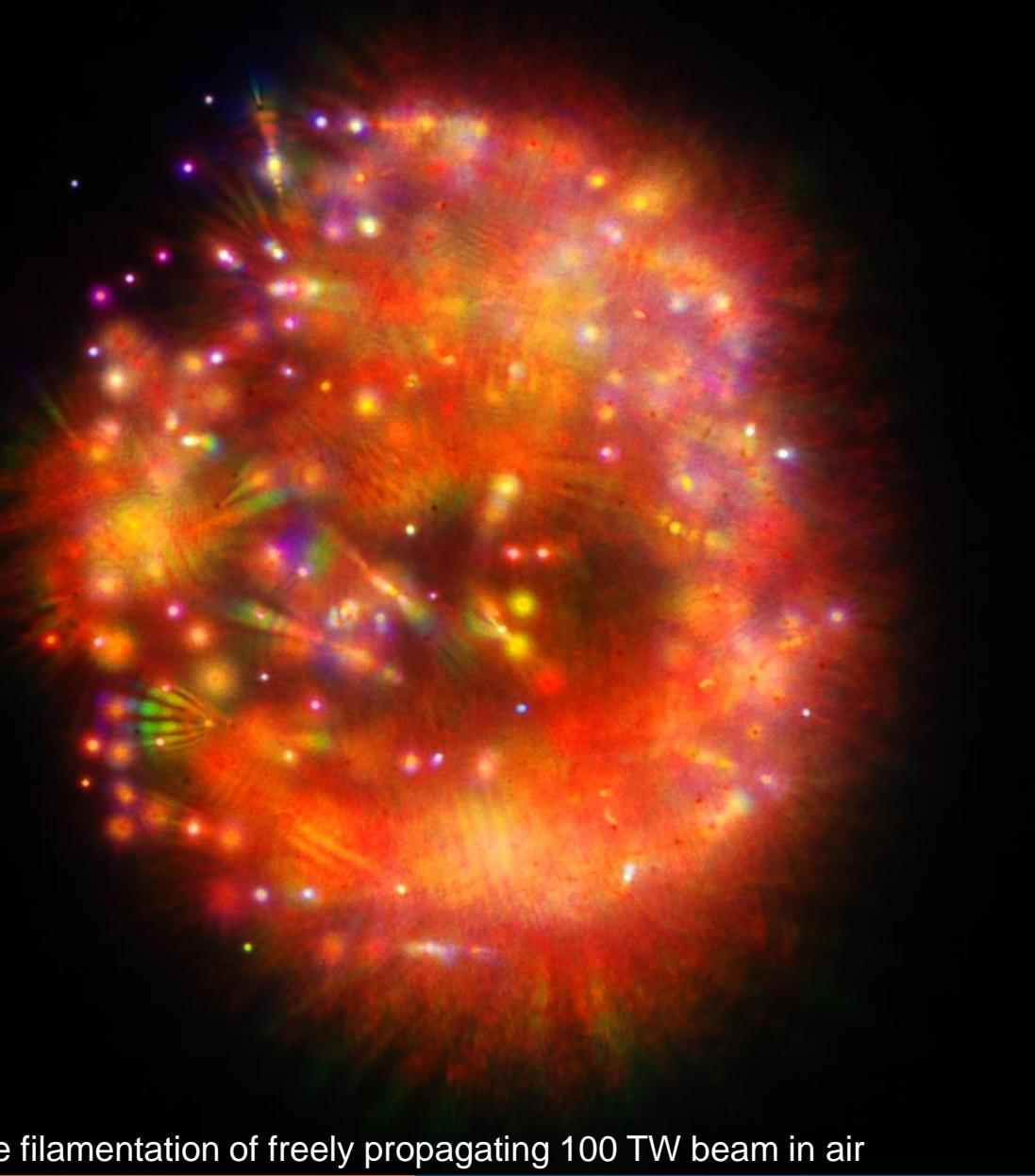
multiple filamentation of freely propagating 100 TW beam in air
