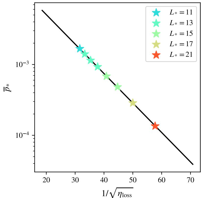
→ “break-even point” (at which  $\bar{p}_* = p = 10^{-3}$ ) occurs at  $\eta_{\text{loss}} = 7.4 \times 10^{-4}$
