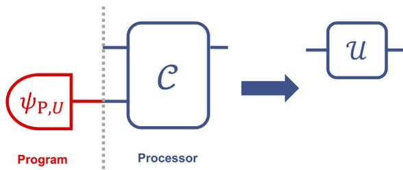
FIG. 1: **An approximate universal quantum processor.** An approximate universal quantum processor executes a unitary gate  $U$  on a system. It works by plugging a quantum state – the program for  $U$  – into the processor, which performs a quantum channel  $\mathcal{C}$  that approximates  $U$  on the system.
