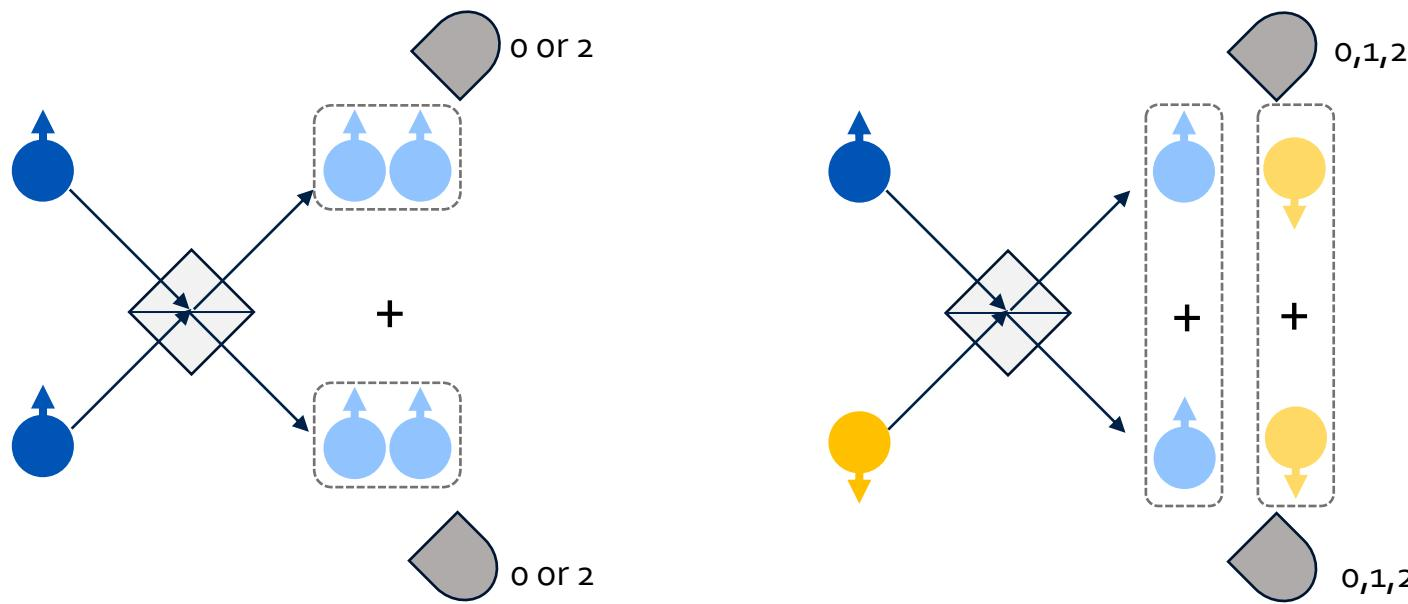
Non-polarising beam-splitter and number counting are able to tell if the polarisations are equal or opposite
